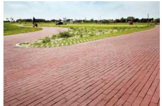
The new UrbanA+ paver, which was specifically developed for pedestrian zones and squares, was used for the footpaths. The pressed clay paver, fired especially hard, is also available in black and violet.
