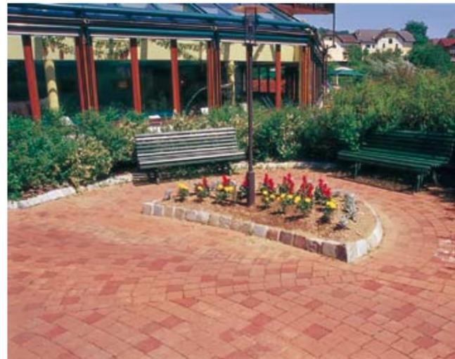
Exit and square design for the "Die Kurzentren" hotel chain, using "Landhaus" pavers with rough surfaces in the colours light red, red, and variegated red. To ensure the best possible drainage, bricks with holes in were used for the parking spaces.
