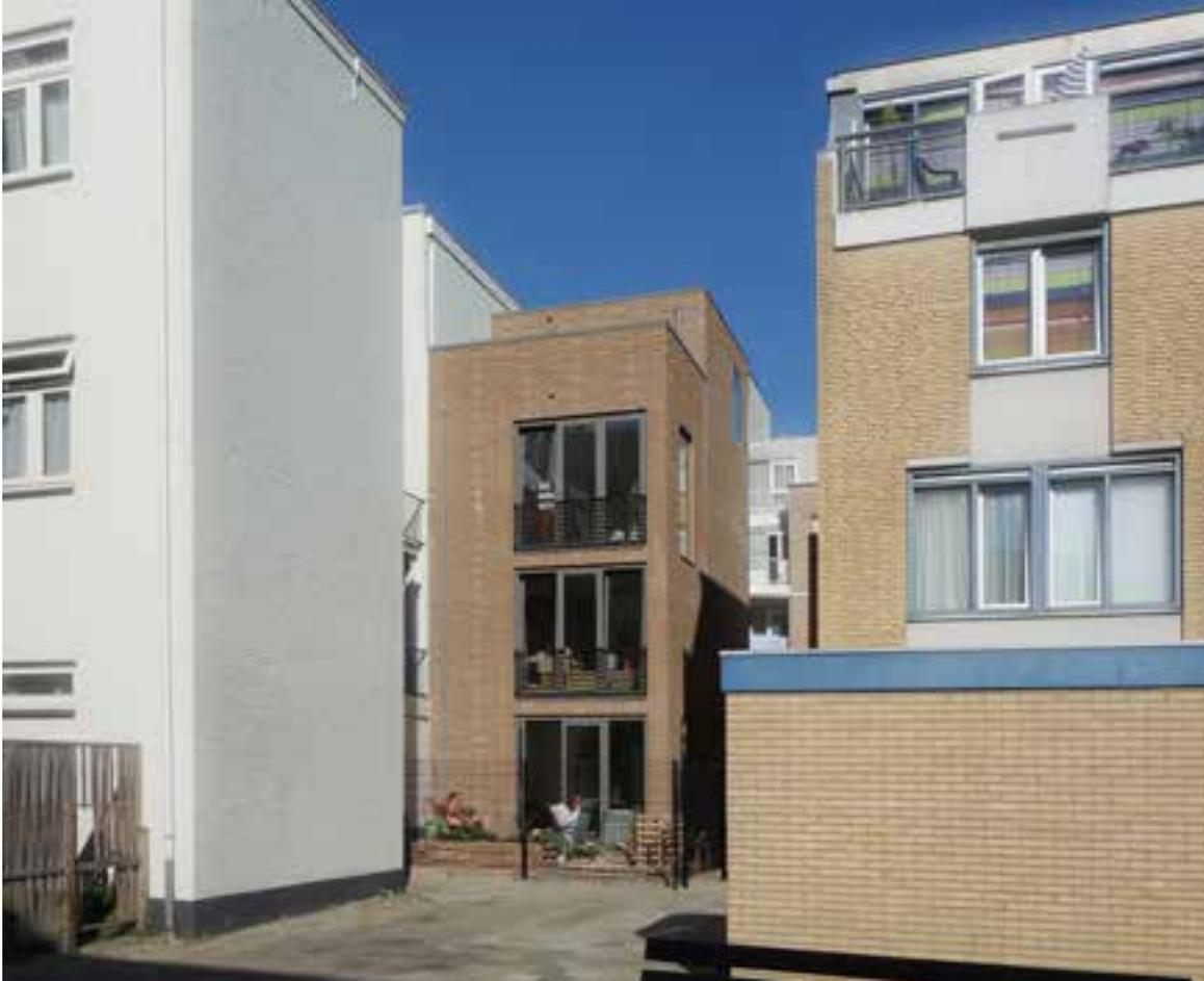
Recycled bricks made of demolition waste were used for the façade.
